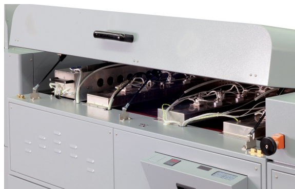
The Infrared Heating System helps cure the water-base and soft-touch varnishing
